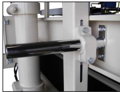
Adjustable Bag Guard Reel to accommodate a full range of bag sizes
