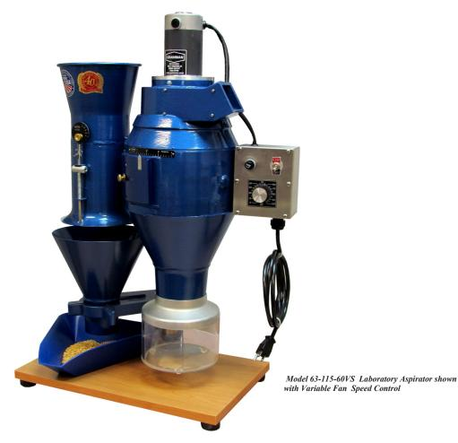
The Grainman Grain Cleaner Laboratory Aspirator Equipment No. 63 is designed for grains and seeds analyst, inspectors and laboratory users who require quick yet thorough separation of granular materials from foreign matter. It can be carried anywhere, requiring small space and may be plugged into any convenient electrical outlet.
